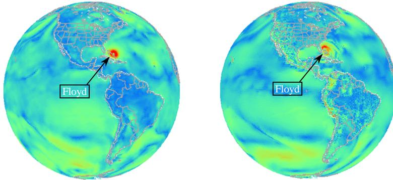
**Figure 7: OMEGA track predictions at 12 hours (left) and 24 hours (right). The grid is adapted to shorelines and the initial hurricane location. Dynamic grid adaptation was not used in this simulation. Pressure perturbation fields are shown in the figure.**
