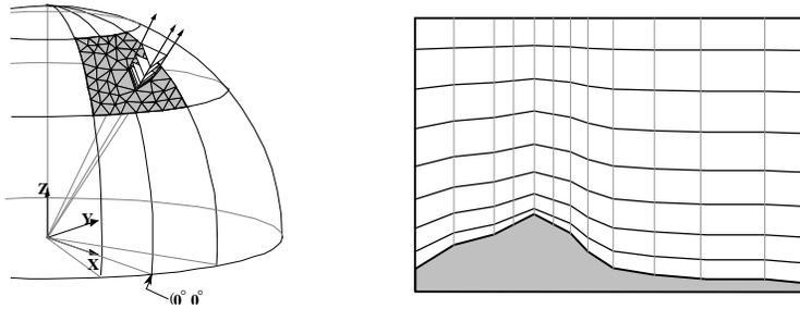
**Figure 4:** The vertical levels of the OMEGA grid are constructed by extending radials through each surface vertex. A set of stretchable layers follow the terrain near the surface and relax to a surface that is parallel to the reference sphere at the top of the grid.
