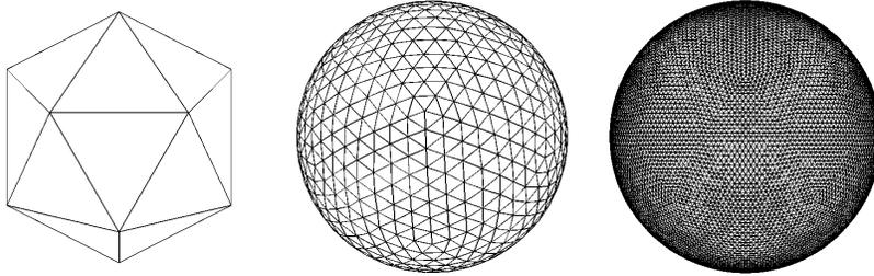
**Figure 1: Initial triangulation (left), mesh after three refinement cycles (middle) and after five refinement cycles (right).**
